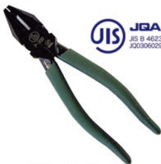
EBP-175 ペンチ 呼び寸法:175mm 重量:290g 切断能力(φmm):銅線/3.2mm 硬線/1.8mm ■Reference Size:175mm ■Weight:290g ■Cutting capacity (φmm): copper wire /3.2mm hard wire /1.8mm
