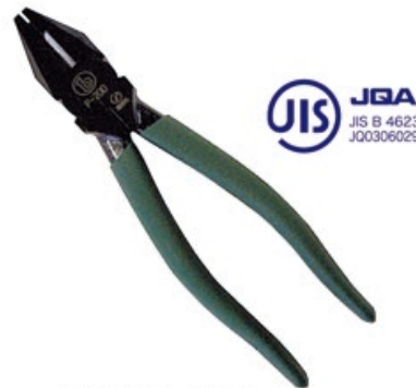
EBP-200 ペンチ 呼び寸法:200mm 重量:390g 切断能力(φmm):銅線/3.2mm 硬線/1.8mm ■Reference Size:200mm ■Weight:390g ■Cutting capacity (φmm): copper wire /3.2mm hard wire /2.0mm
