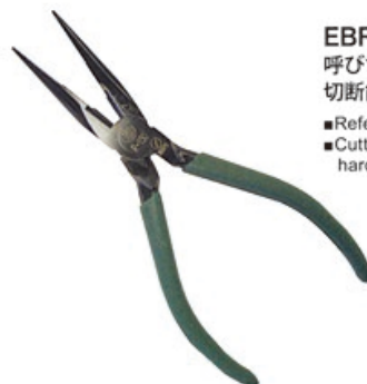
EBP-175 ペンチ 呼び寸法:175mm 重量:290g 切断能力(φmm):銅線/3.2mm 硬線/1.8mm ■Reference Size:175mm ■Weight:290g ■Cutting capacity (φmm): copper wire /3.2mm hard wire /1.8mm
